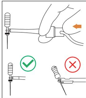
c) In apex locator mode it is suggested to install the motor handpiece in the charging base to get better visual angle.
