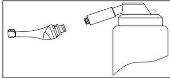
3. Fill the contra-angle with oil until the oil flows out of contra-angle head part.
