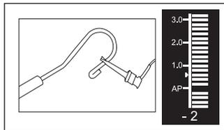
2. In combined Motor and Apex locator mode, touch the lip clip with the file and check that all the indicator bars light up, as shown below:
