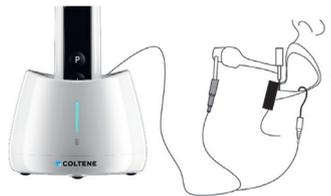
d) The Apex locator detects the canal apical foramen, not the tooth anatomical apex. This could explain some differences between the apex locator signal and an X-ray image.
